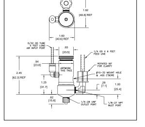
The amount of fluid that flows through the valve is determined by: (1) length of time the valve is open, (2) fluid reservoir pressure, (3) output dispensing tip size, (4) diaphragm stroke and (5) fluid viscosity. The Loctite® 98009 Light Cure Valve may be used for a wide range of applications. Henkel recommends that you test all adhesive applications under simulated or actual end use conditions to ensure the adhesive meets or exceeds all required production specifications.
