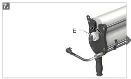
Remove cartridge nose plug (E) by turning retaining nut 120 deg counterclockwise.
